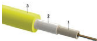
1. Dry tube with optical fibers 2. Water-blocking e-glass yarn 3. FRLSZH outer sheath
