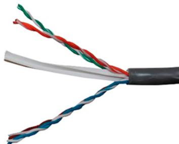
Category 6 U/UTP Cable, 24AWG, low smoke zero halogen, gray jacket, 4 pair count, 305 m length Reel in box
