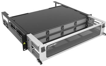
High Density 2U Sliding Fiber Splice Panel, to accommodate a maximum of 96 single fusion splices when using the Splice Wallet® or 64 single fusion splices when using the RoloSplice® splice tray organizers
