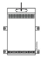
3. **Connect ground terminal first**. Then connect the remaining wires. Route wires through the knockout hole to the terminal blocks. See diagram below. Refer to "Wiring Specifications" on page 1.
