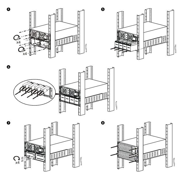
The process for installation of an external battery pack with UPS models SRT8K/SRT10K models is identical to that described for the SRT5K/SRT6K models.
