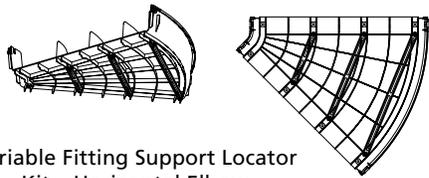
Variable Fitting Support Locator Kit – Horizontal Elbow
