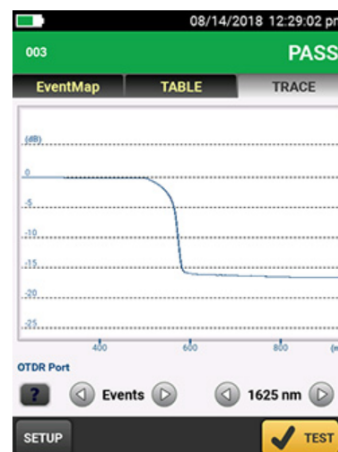
Splitter as seen on an OTDR trace
