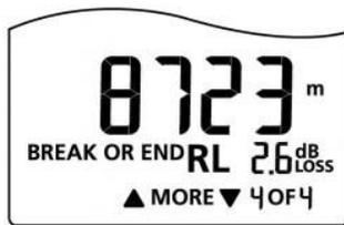
The result loss of the fiber (RL) is 2.6 dB.
