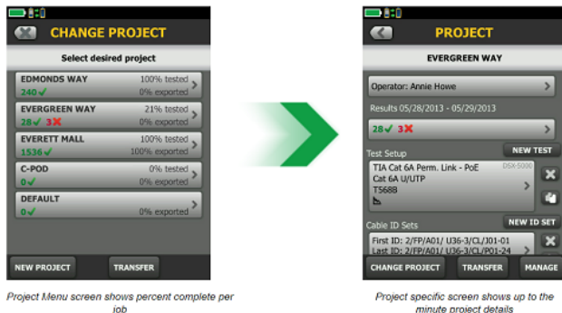
Project Menu screen shows percent complete per job
