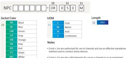
Cords < 1m are also valid elements for use in a channel or as an equipment interconnect but due to their limited length are not guaranteed to meet component compliance requirements that were developed to assess the quality of longer cords
